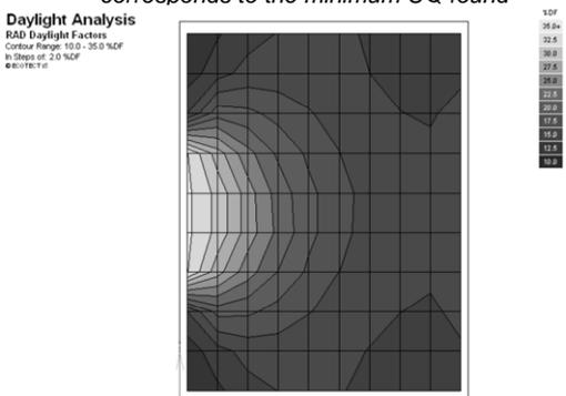
Fig 10. Simulation made to the to the window positioned on the 4m wall (variation on environment geometry), situation that corresponds to the maximum UQ found
