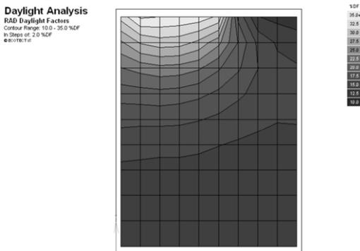
Fig 9. Simulation made to the window positioned on the left (variation on windows' position), situation that corresponds to the minimum UQ found
